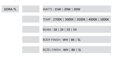
15w-1600lm | 20w-2280lm | 30w-3250lm (Based on 3000k)
